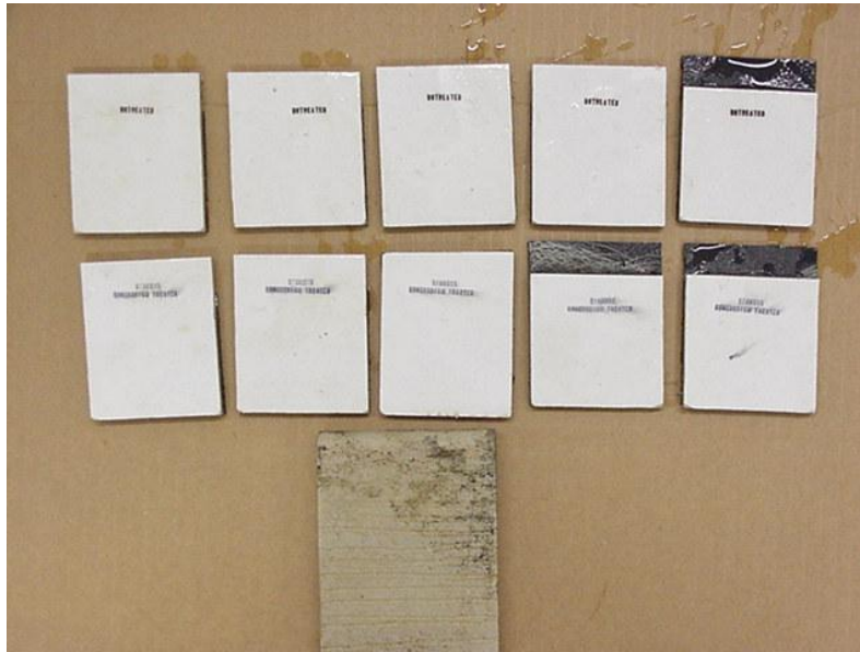
Figure 2 Week 6 Samples (Upper Row – Untreated; Lower Row – Treated) Bottom – a control board from the same ASTM Cabinet
